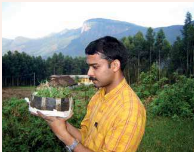
Transpiration from the grasslands being measured using a simple lysimeter.
