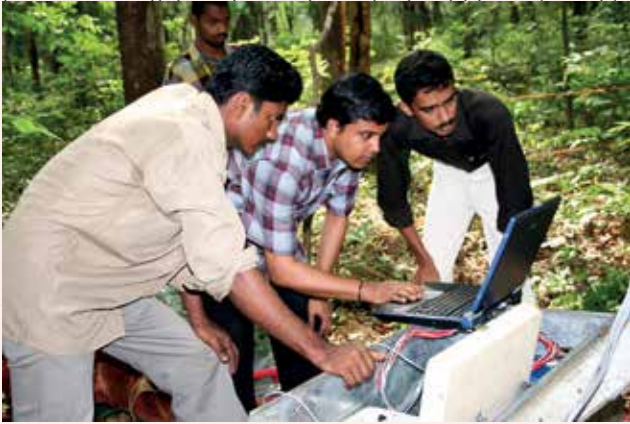
Sapflow velocity being monitored in a field computer attached to the sapflow system on the eucalypt trees.
