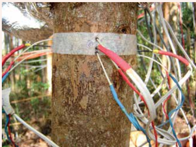
Sapflow measurements being done in a eucalypt tree trunk to understand the water consumption. Sensors and heat pulse generators are inserted into the wood to measure the velocity of sap flow.
