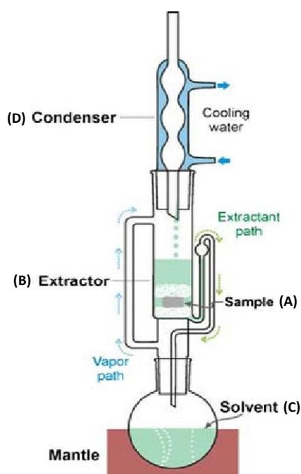
Figure -3.1 Soxhlet apparatus
