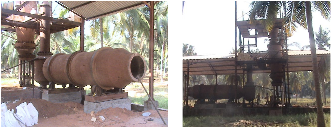
Fig. 6. Newly developed RFBR Shell Charcoal Activation Plant
