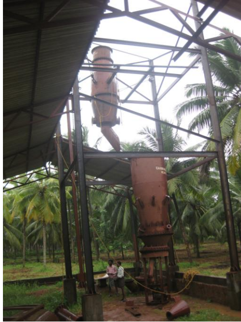
Fig. 3. Vertical carbonizer with coconut shell dryer
