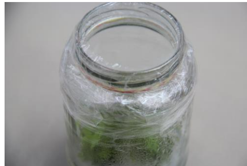
Figure 2. Clear transparent closures made of PP sheets
