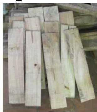
Fig. 21. (a) Surface growth on open stacked control rubberwood blocks in the summer season after one month of incubation (b) Inhibition of fungal growth on close stacked rubberwood blocks treated with Bacillus subtilis B1 culture
