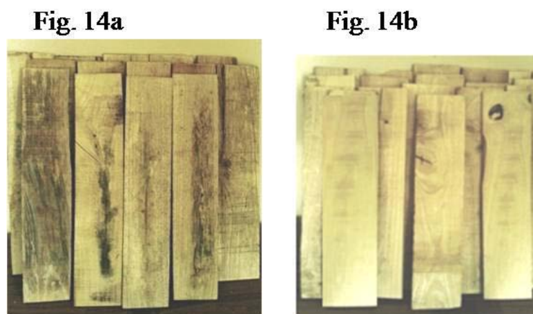
Fig. 14. (a) Internal stain on close stacked control rubberwood blocks in the Northeast monsoon after one month of incubation (b) Absence of internal stain on close stacked rubberwood blocks treated with Bacillus subtilis B1 culture after one month of incubation
