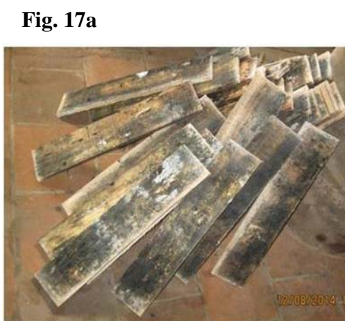
Fig. 17. (a) Surface growth on close stacked control rubberwood blocks in the Southwest monsoon after one month of incubation (b) Inhibition of fungal growth on close stacked rubberwood blocks treated with Bacillus subtilis B1culture
