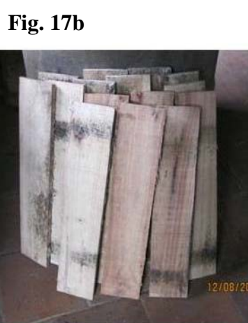
Fig. 17. (a) Surface growth on close stacked control rubberwood blocks in the Southwest monsoon after one month of incubation (b) Inhibition of fungal growth on close stacked rubberwood blocks treated with Bacillus subtilis B1culture
