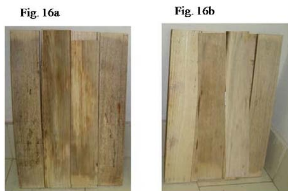
Fig. 16. (a) Internal stain on close stacked control rubberwood blocks during the summer season after one month of incubation (b) Absence of fungal growth on close stacked rubberwood blocks treated with Bacillus subtilis B1culture
