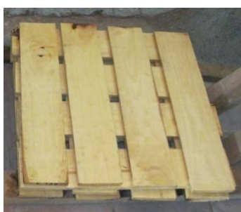
Fig. 3. Open stacking of rubberwood blocks
