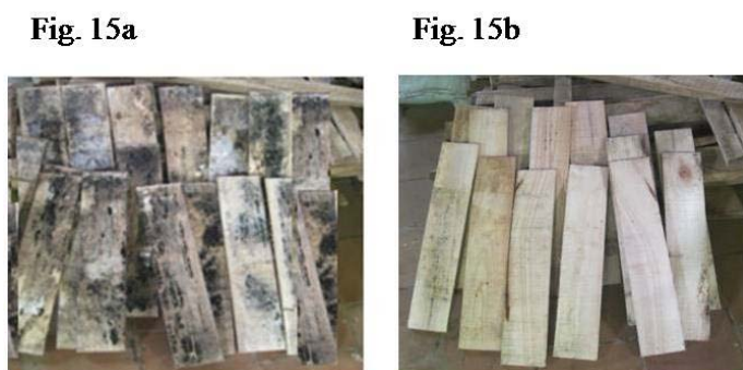
Fig. 15. (a) Surface growth on close stacked control rubberwood blocks during the summer season after one month of incubation (b) Inhibition of fungal growth on close stacked rubberwood blocks treated with Bacillus subtilis B1 culture during summer season
