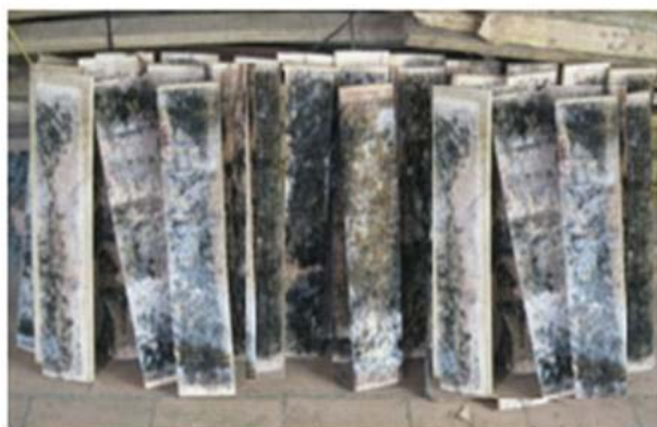
Fig. 13. (a) Surface growth on close stacked control rubberwood blocks in the Northeast monsoon after one month of incubation (b) Inhibition of fungal growth on close stacked rubberwood blocks treated with Bacillus subtilis B1 culture
