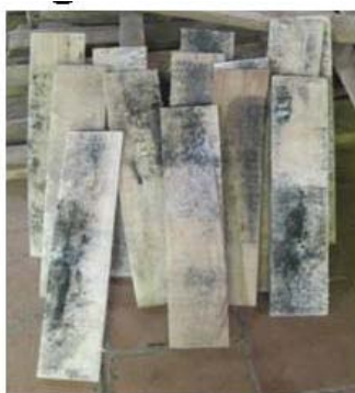
Fig. 21. (a) Surface growth on open stacked control rubberwood blocks in the summer season after one month of incubation (b) Inhibition of fungal growth on close stacked rubberwood blocks treated with Bacillus subtilis B1 culture
