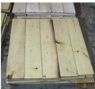
Fig. 2. Close stacking of rubberwood blocks
