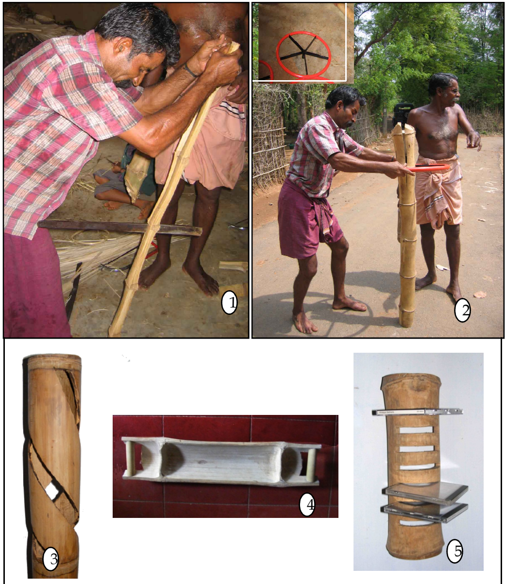
Fig 4. 1. Traditional way of splitting 2. splitting using new wheel-like tool. 3. Design of a lampshade 4. fruit tray and 5 CD rack
