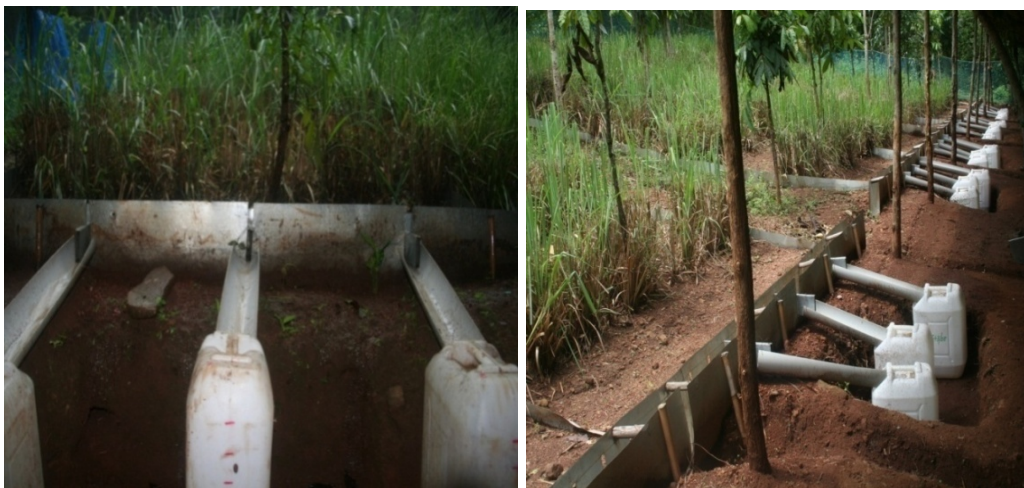
Fig.3. The process of runoff collection through multislot divisors
