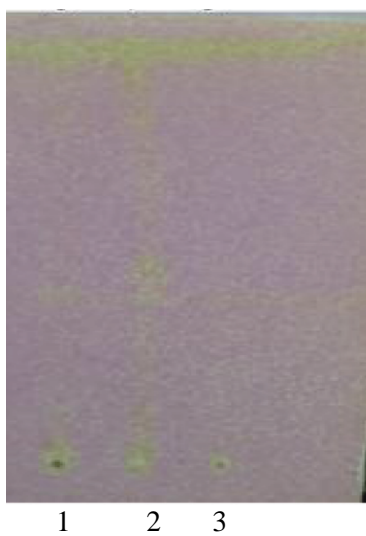
Figure 8. TLC analysis of acetone extract of Kaempferia rotunda and substitutes with the solvent system, ethyl acetate: benzene (9:11). Plate sprayed with spray reagent 0.2% aqueous potassium permanganate. Lane 1. Lagenandra ovata , 2. Lagenandra toxicaria and 3. Kaempferia rotunda
