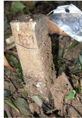
Fig. 9 Wood stake attacked by termites
