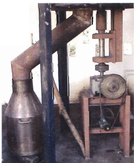
Fig 17.Outlet pipe fitted to the product withdrawal cane & motor assembly to push out the charcoal
