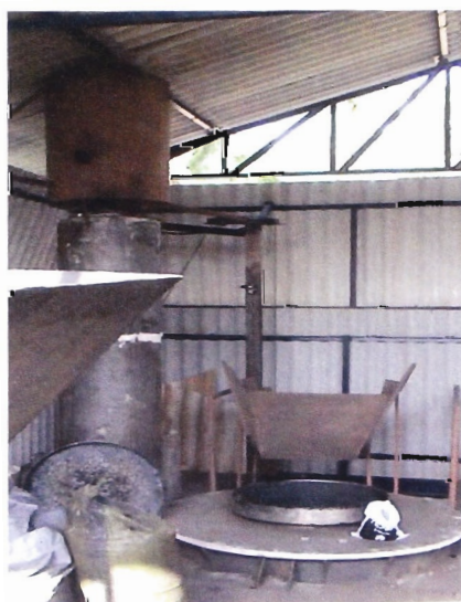
Fig 18. Flue gas burning furnace, attached to the chimney; and feeding hopper
