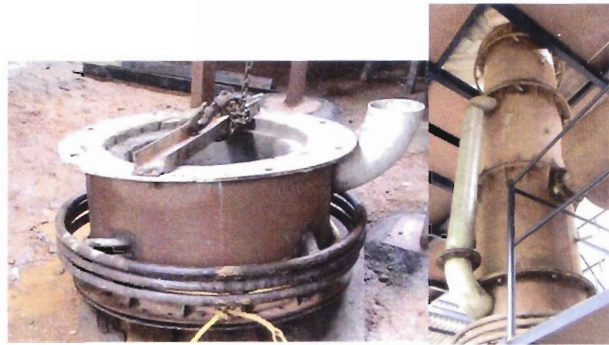
Fig. 35. Bottom (4 th ) chamber with three rings (note the overall view of bottom chamber with three rings for air, steam and LPG as well as the heat exchanger between 2 nd & 4 th chambers)
