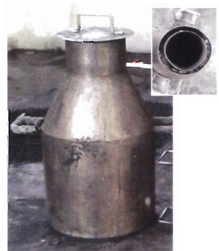
Fig. 22. Charcoal collection can; (note the water jacket portion in the neck of the can)
