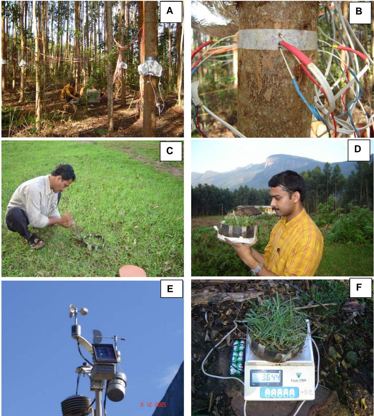
**Plate II.** A. Sap flow of eucalypt trees being measured using the sap flow sensors. B. Close up of a tree trunk fixed with sap flow sensors and the heaters. C. Fixing a small weighing lysimeter in the grassland at Kanthalloor. D. A weighing lysimeter with a patch of grassland in it. E. An automated weather station installed near the eucalypt plantation at Kanthalloor. F. The small lysimeter being weighed on a field electronic balance.
