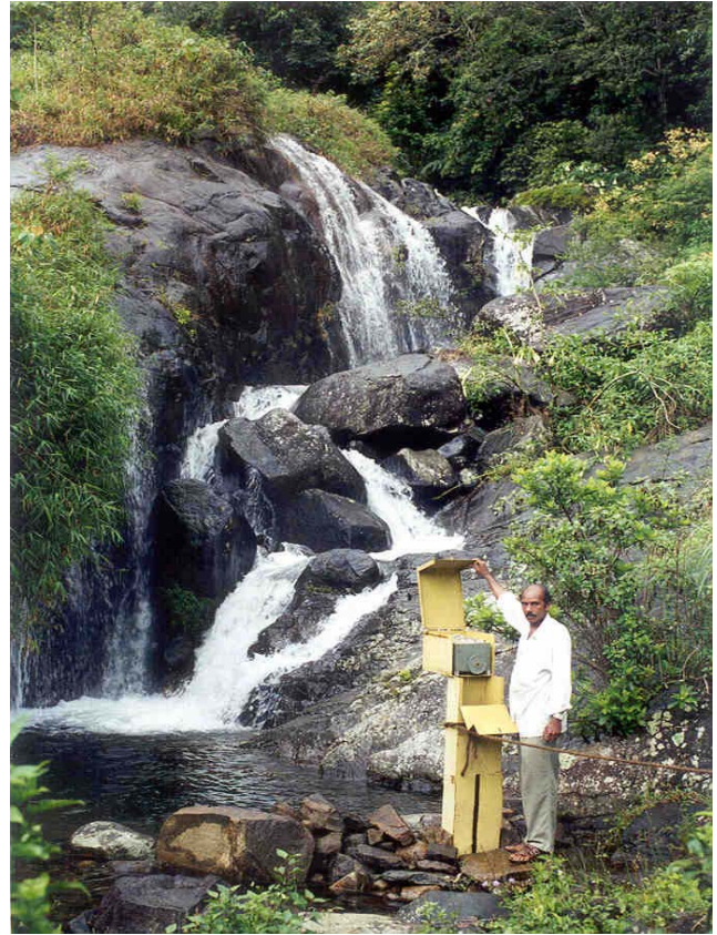
Pl.5.A view of the stream section in catchment 1 showing the stage level recorder and stilling well
