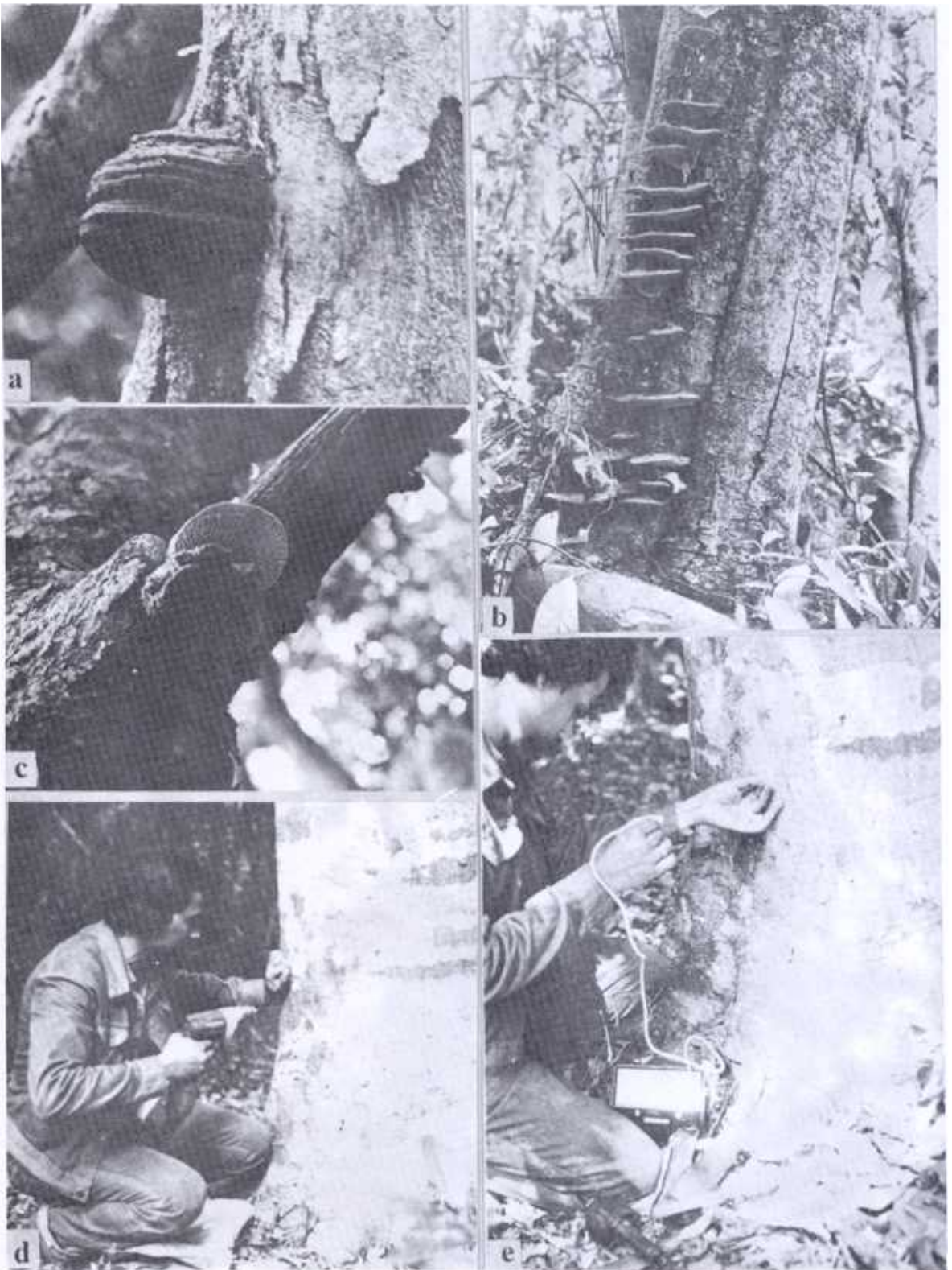
Fig.3.a-c: Tree showing decay indicators (sporophores of decay fungi) a,b: trees exhibiting sporophores of Phellinus spp. on top (a) and basal parts of the trunk. c: Fruticification of Lenzites sp. on the decayed branch. d-e: detection of decay by measuring the electrical resistance of the wood; d: drilling the probe hole using battery operated drill; e: recording the electrical resistance of the wood using Shigometer.
