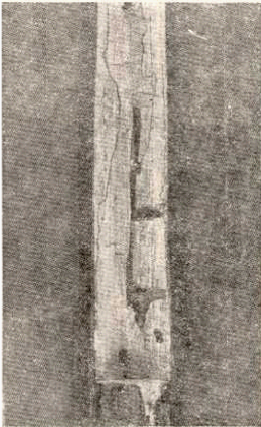
Fig. 1. Gmelina arborea in longitudinal section showing tunnels made by Acalolepta rusticatrix .
