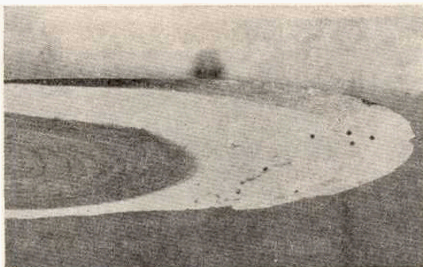
Fig 8 — Plank of Dalbergia latifolia showing damage caused by Sinoxylon anale to the sapwood.
