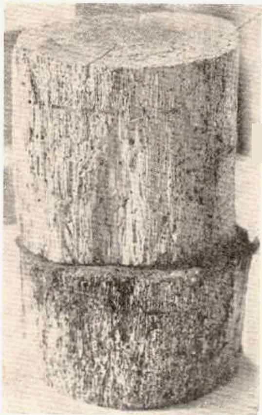
Fig. 4 — Round logs of Bombax ceiba heavily attacked by Sinoxylon anale .
