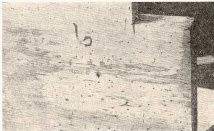
Fig. 3 — Plank of Artocarpus heterophyllus showing pinholes of Xyleborus similis .
