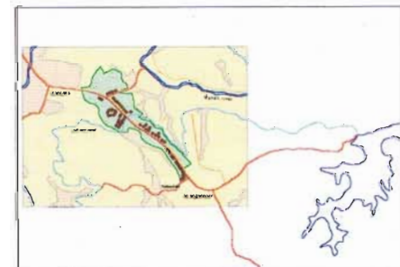
Bit map prepared for the purpose of overlaying on the three-d map. The map of exactly same coordinates as the area digitized for contours was made in Mapinfo as vector lines and polygons and converted to bitmap.
