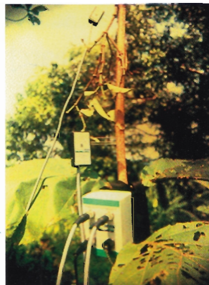
A sap flow gauge fixed to a teak tree is used to monitor the transpiration in the tree. The datalogger stores the data at programmed intervals.
