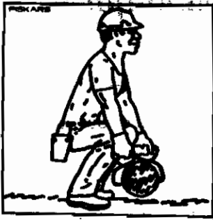
Fig. 3. Use a correct lifting technique. Keep your back straight. The strong leg muscles will do the lifting.
