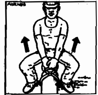
Fig. 10. Use tongs and grip. Place on top of leg muscles for lifting.
