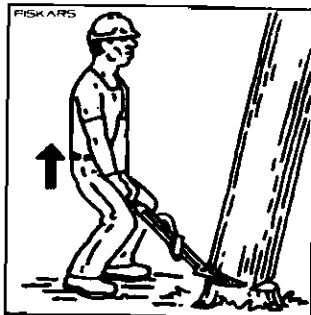
Fig. 20 Use your leg muscles and keep your back straight. When tilting with the felling lever.
