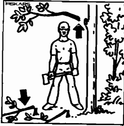
Fig. 6 Cut the bushes and lower branches to clear a safe working space; Take a steady leg spread position for efficient and safe working.
