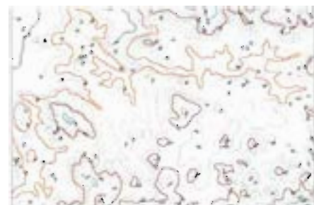
The contour lines digitized at 20 m interval is colour coded for clarity.
