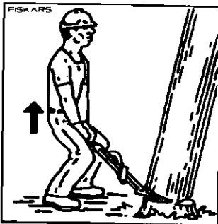
Fig. 20 Use your leg muscles and keep your back straight. When tilting with the felling lever.
