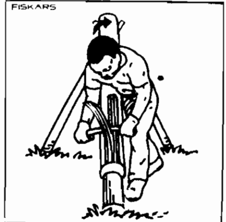
Fig. 12. Turn the log around towards yourself and use pushing strokes.
