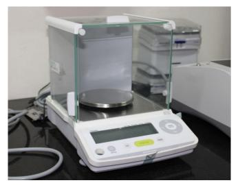
Weighing balance is used to calculate the weight or mass of an object/chemicals used for plant culture. It tissue has higher readability, measuring to the nearest 0.0001 g, drought-proof camber and anti-vibration tables which enable high accurate measuring. Precision balance has a resolution near 0.1-
