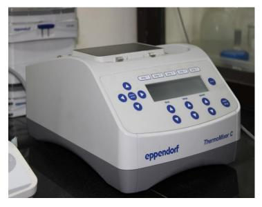
Thermo Mixer (Microbial hot mixer) is a device for the temperature control and mixing of liquids or samples. The device offers a wide temperature control range (1 °C–100 °C), high flexibility with the use of diverse tube and plate formats and advanced mixing performance with a mixing speed of 3000
