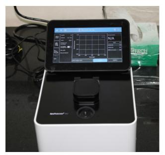
The NanoDrop Spectrophotometer is a simple, easy-to-use spectrophotometer for measuring DNA, RNA, and protein concentrations in small volume samples. The instrument operates by passing a beam of light through a sample and measuring the intensity of light reaching a detector employing Beer's law. 1 ul sample is pipetted onto the end of a fiber optic cable (the
