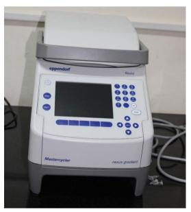
The thermocycler is a laboratory apparatus most commonly used to amplify segments of DNA via the polymerase chain reaction (PCR). Most models have a gradient function to allow for different temperatures in different parts of the block. The PCR process is conducted via thermal cycling, a process of heating and cooling that creates the conditions necessary for DNA replication.
