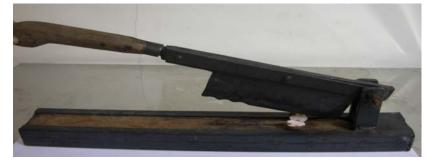
Fig. 32. A heavy duty seed cutter used for cutting test of teak seeds.
