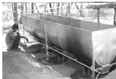
Fig. 3. Nomad type Cane Curing Unit for field demonstration at KFRI Sub-Centre, Nilambur, Kerala
