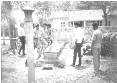
Figure 2. The mud-hearth type design of the cane curing system, using firewood as the heat source
