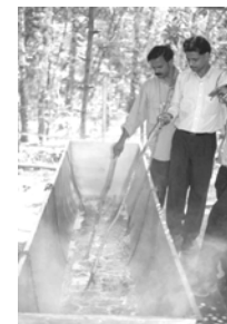
Fig. 3. Nomad type Cane Curing Unit for field demonstration at KFRI Sub-Centre, Nilambur, Kerala
